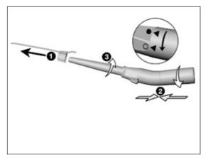
Disassemble angled handpiece S-9 L G, S-9, S-10, S-12, S-16
