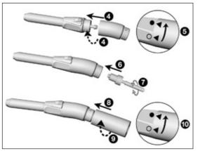
Push the shaft into the handpiece head. Insert the knee onto the handpiece head.
