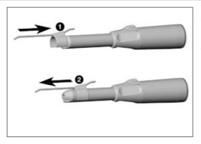
Coolant tubeFit the coolant tube.
