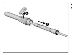
4 Remove the chuck lever.
