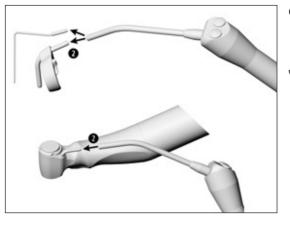
2 Blow through the coolant tube and coolant outlets using compressed air.
